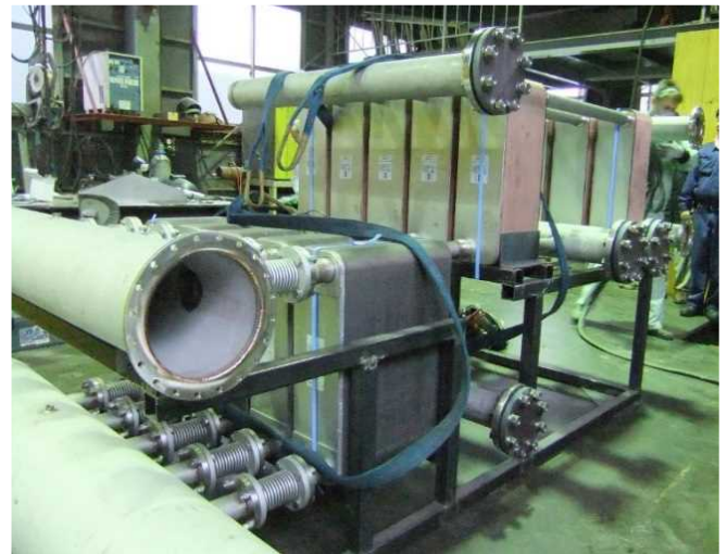
Fig 4-3 The Heater, the Cooler and the Regenerator system
