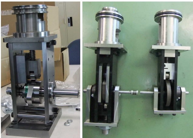
Fig 5-2 Floating Valve-Seat type Poppet Valves
